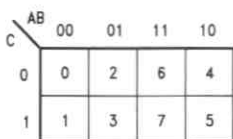
FIGURE A.4.5. K-Maps for Two and Three Variables
