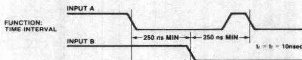
Figure 3: Waveform for Minimum Time Between Transitions of Input A and Input B.
